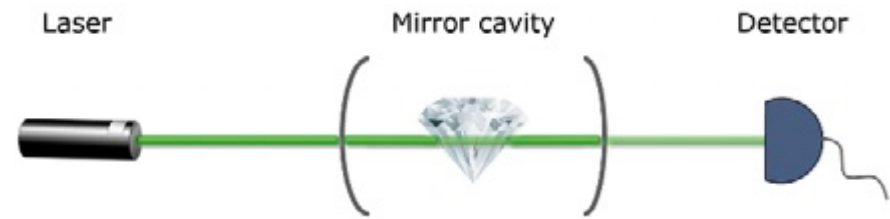
Figure 5, Simple sketch of the experimental set-up. The diamond containing NV centres sits in a cavity between two mirrors. A laser shines green light into the cavity where it bounces back and forth and passes through the diamond many times. On the other side of the cavity, a detector measures how much of the light the diamond absorbed.
